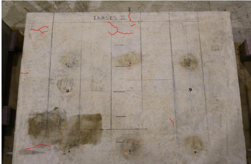
Figure 76. Visible cracking in south portion of slab 2 (top) and north portion of slab 1 (bottom).
