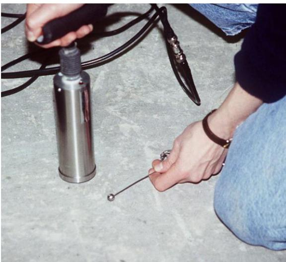
Figure 7. Impact echo setup with a steel ball mounted on a steel spring rod (Carino, 2001).
