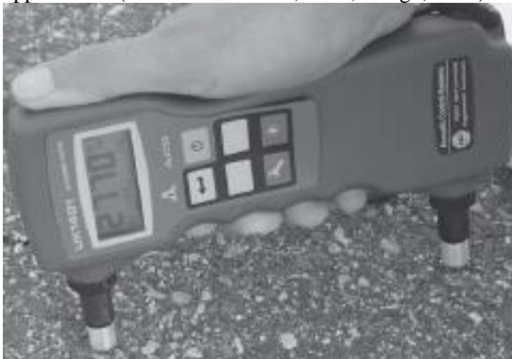
Figure 10. UK1401 ultrasonic pulse velocity device (Khazanovich et al., 2005)
