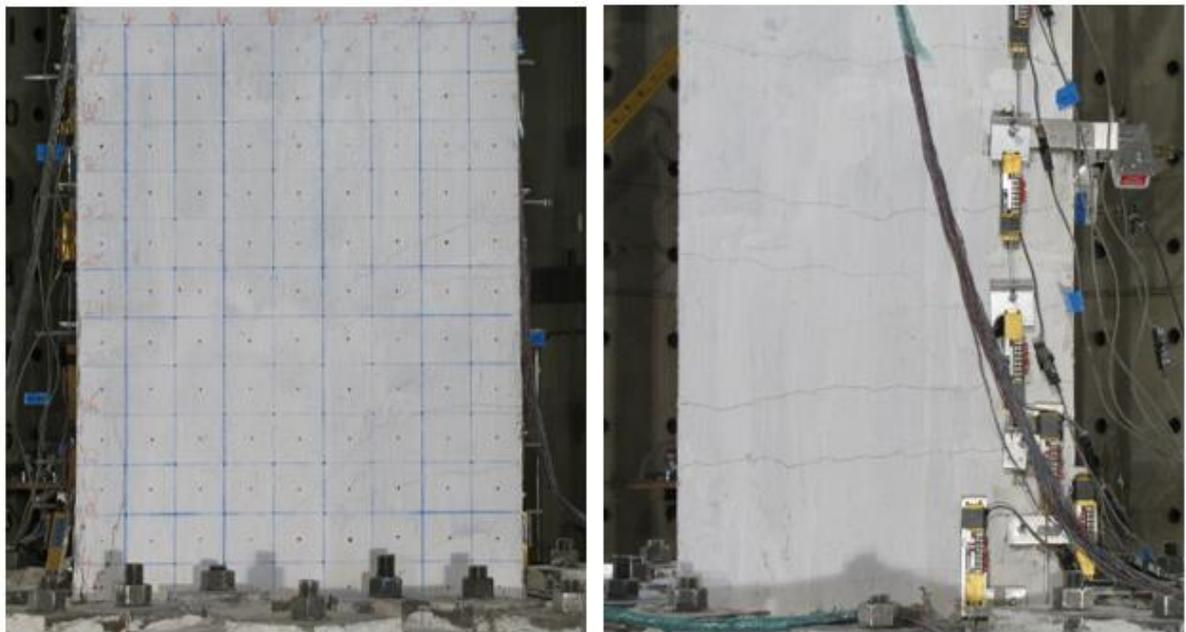
Figure 43. Column condition for 3rd set of MIRA measurements (after 1% drift ratio was attained).
