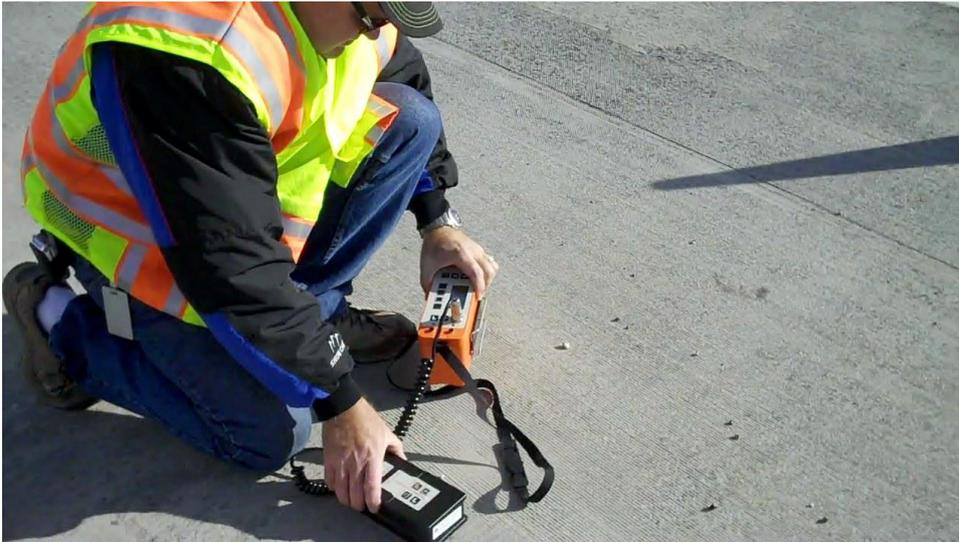
Figure 3. Pachometer: a magnetic pulse-induction device and its application on concrete pavement (adapted from Hoegh, 2013)
