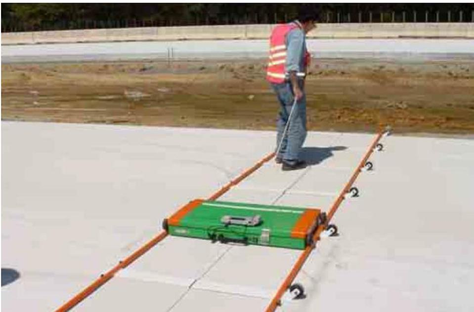
Figure 4. MIT Scan-2: a magnetic pulse-induction device and its application on concrete pavement (adapted from Yu et al., 2005)
