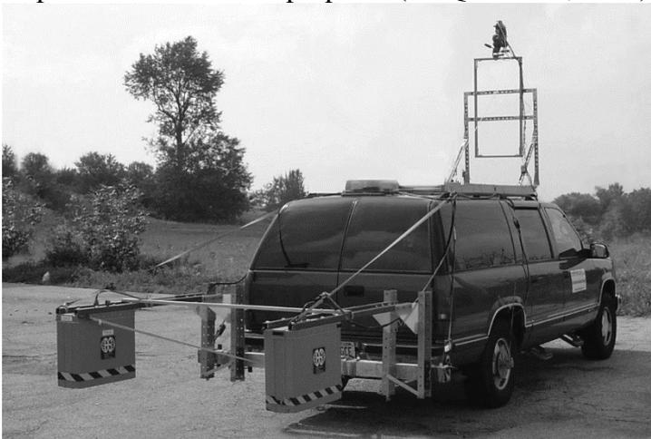
Figure 6. Air coupled GPR mounted on a van for highway speed measurements (Maser, 2000).
