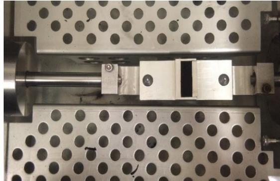
Figure 3-6 Tensile adhesive method fixture in the bath before testing.
