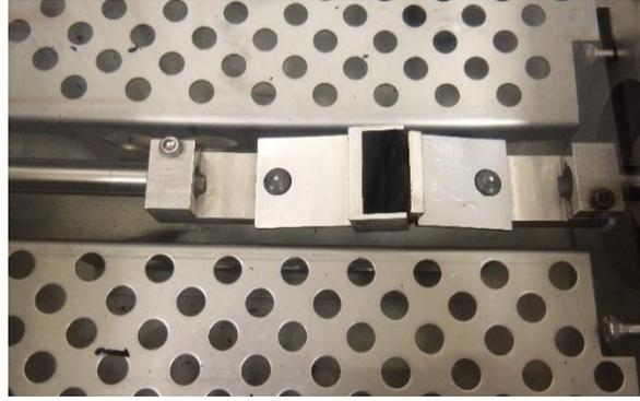
Figure 3-7 Tensile adhesive method fixture after failing.
