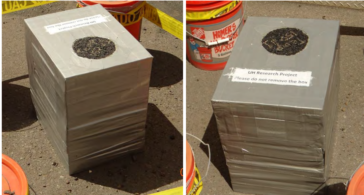
Figure 5-4 Styrofoam box with HMA, granular base, and datalogger used to collect mix temperatures with depth.
