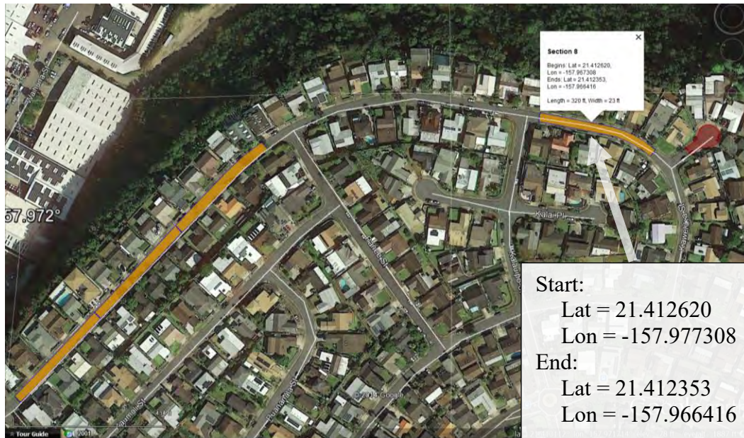
Figure A-11 Location of Section 8 on Kaweloka Street – Control Section for Seal Coats with no bus loading.
