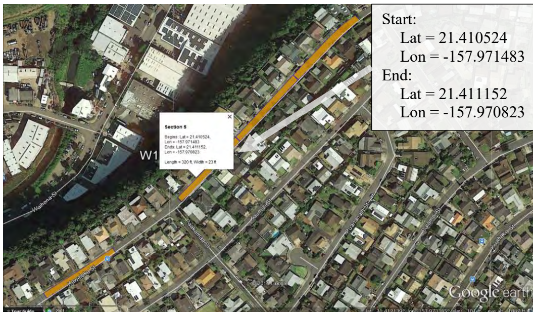
Figure A-8 Location of Section 5 on Kaweloka Street – Seal Coat with “CarbonSeal-HF” by GP Roadway Solutions.
