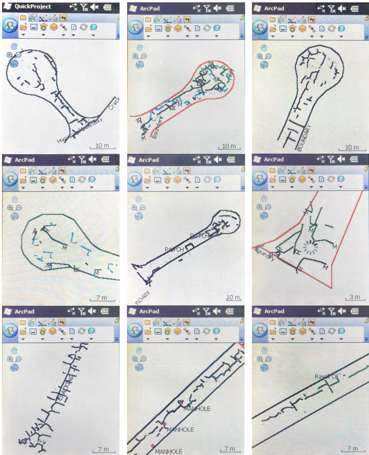
Figure 4-1 Examples of initial efforts to quantify distresses with a handheld GPS.
