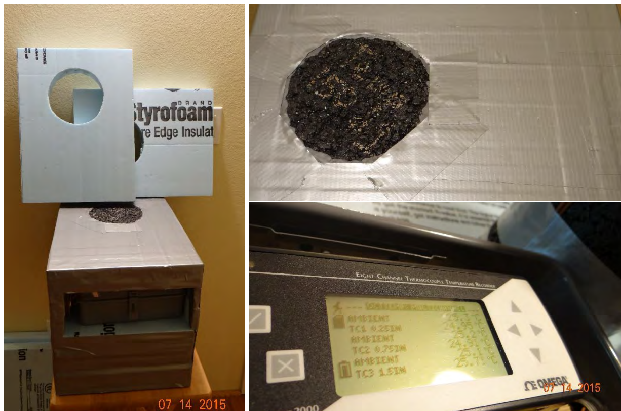
Figure 5-3. Styrofoam box setup used to monitor pavement temperature with depth.
