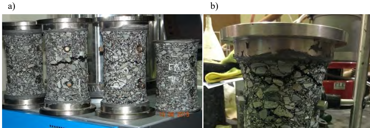
Figure 6-6 Successful middle breaks (left) and unsuccessful end breaks (right).
