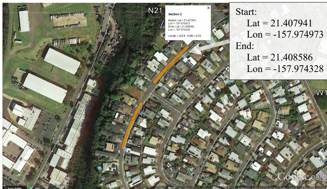
Figure A-6 Location of Section 3 on Kaweloka Street – Seal Coat with “MasterSeal™ Ready to Use (Asphalt Based Pavement Sealer Fortified with Gilsonite)” by SealMaster®/Hawaii.
