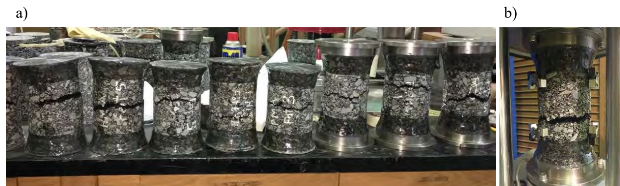
Figure 6-8 Effectiveness of specimen configuration to induce mid-specimen fracture.
