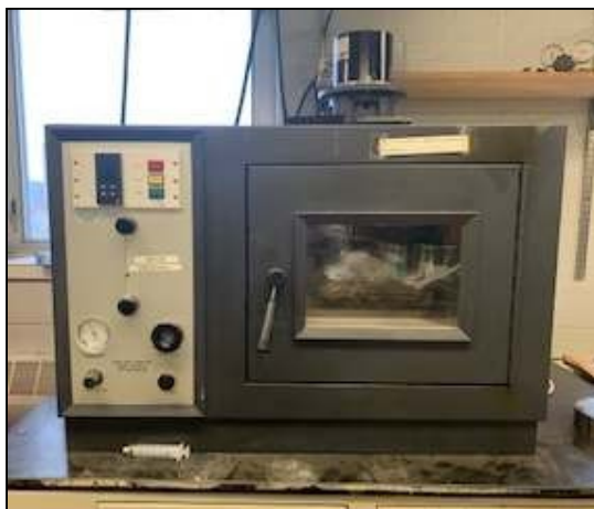
Figure 3.9-Rolling Thin Film Oven
