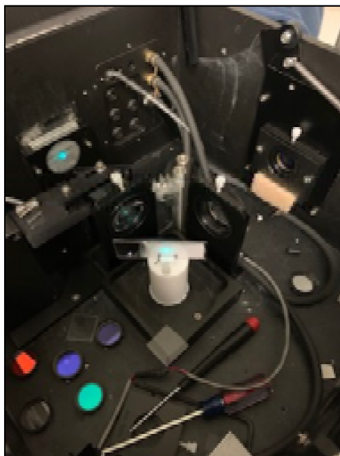
Figure 3.11- Photoluminescence Spectrometer Sample Component
