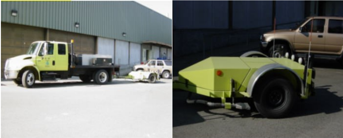
Figure 2-7 (left) Locked-wheel skid tester and (right) trailer
