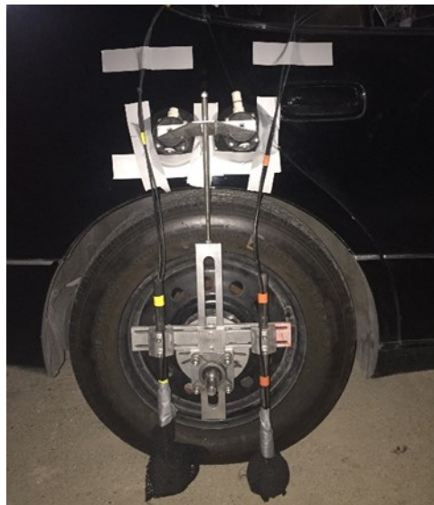
Figure 4-10 OBSI dual probe configuration setup
