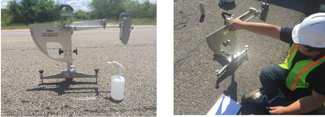
Figure 2-4 (left) BPT and (right) field operation
