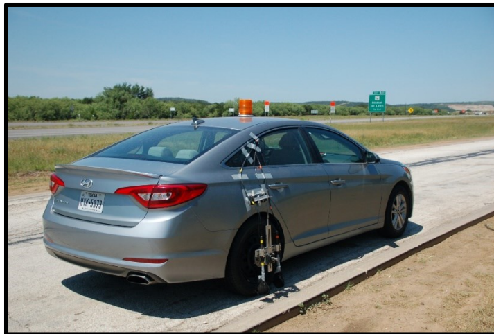
Figure 5-2 OBSI setup on passenger side rear wheel
