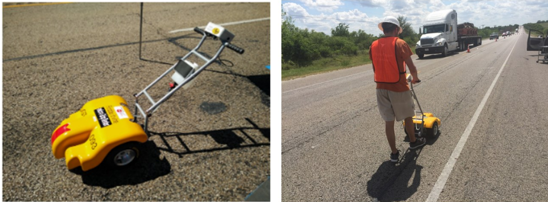
Figure 2-6 (left) Micro-GripTester device and (right) field operation
