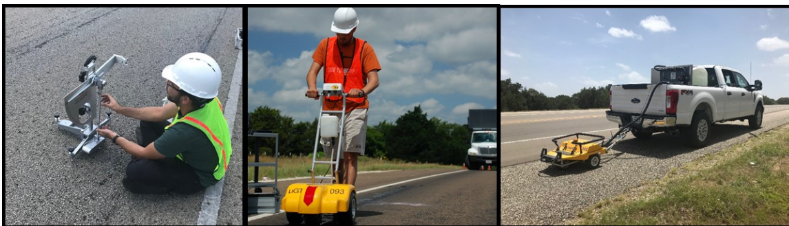
Figure 5-4 (left) BPT in operation, (middle) micro-GripTester, (right) GripTester attached to vehicle
