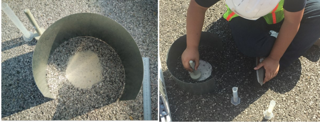
Figure 3-8 (left) SPT equipment, and (right) field data collection
