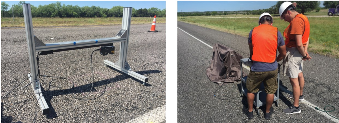
Figure 3-12 (left) LLS and (right) field operation
