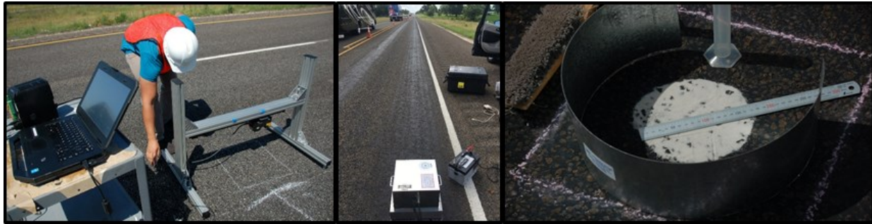
Figure 5-3 (Left) LLS in operation, (middle) CTM placement, (right) SPT
